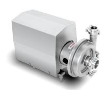
The pump body and impeller adopt the whole fine casting and good part surface treatment. The shaft seal adopts an open structure, so it can be observed in time even if there is a small leakage at the shaft seal. It will not overflow into the motor even if it is not noticed for a short time. Thus, the service life of the motor is guaranteed.
