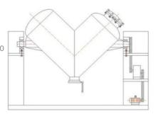
The inner wall of the container needs to be polished to make the inner surface very smooth, so that the powder and granules can flow fully, and it is also conducive to discharging and cleaning. The lengths of the two barrels of the V blender are not equal, in order to more effectively disrupt the movement of the material in the mixing chamber, increase the degree of "turbulence", and facilitate the full mixing of the material.
